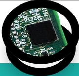
Google's purpose-built chip to establish **hardware root of trust**
